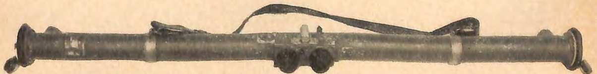
Figure 297. One meter base stereoscopic range finder. The reticle of this instrument is graduated from 250 to 6,000 (presumed to be meters). Markings indicate an 8^\circ\times magnification, a 4.5^\circ vertical and 5^\circ horizontal field of view.
